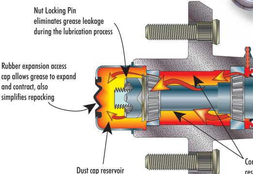
Easily accessible grease channel with grease fitting
