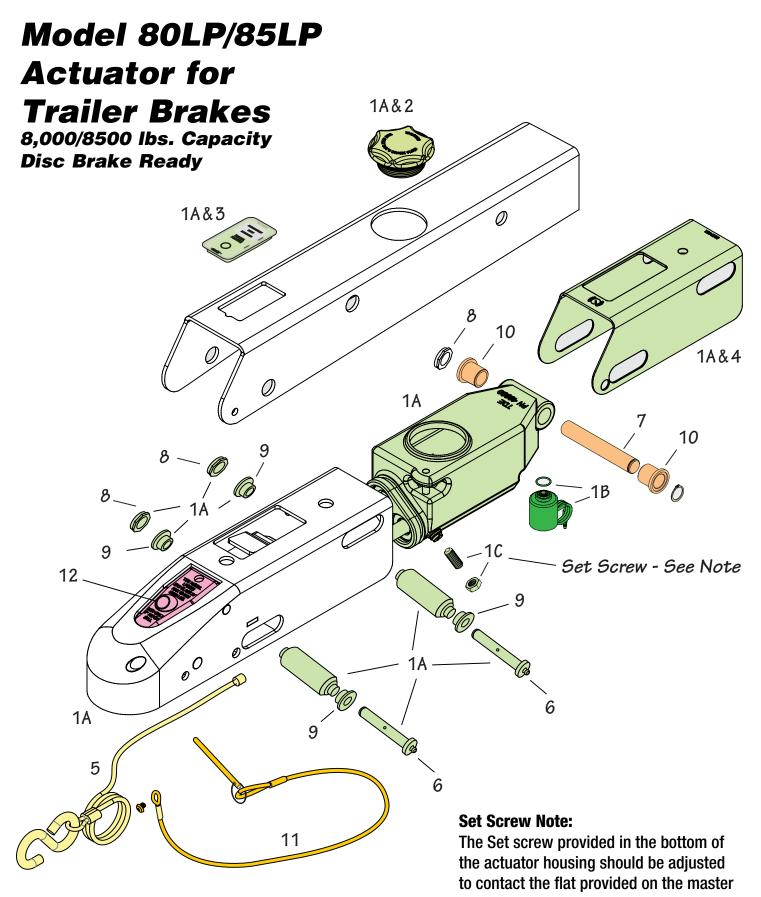
cylinder casting then backed off 1/4 turn and locked in that adjusted position by tightening the jam nut provided.
