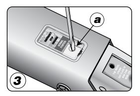
**To Release the Emergency Brake:** Press down the emergency stop release bracket with a screwdriver (#3-a) until the E-stop bracket snaps back into the "NORMAL POSITION" (#1).
