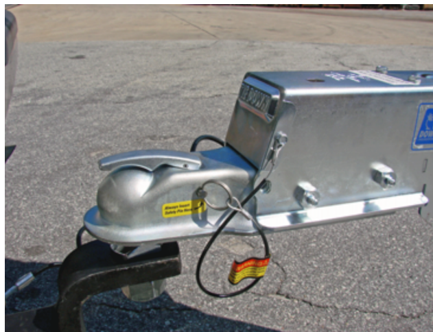
Photo B – Latch Closed, Safety Pin Installed
