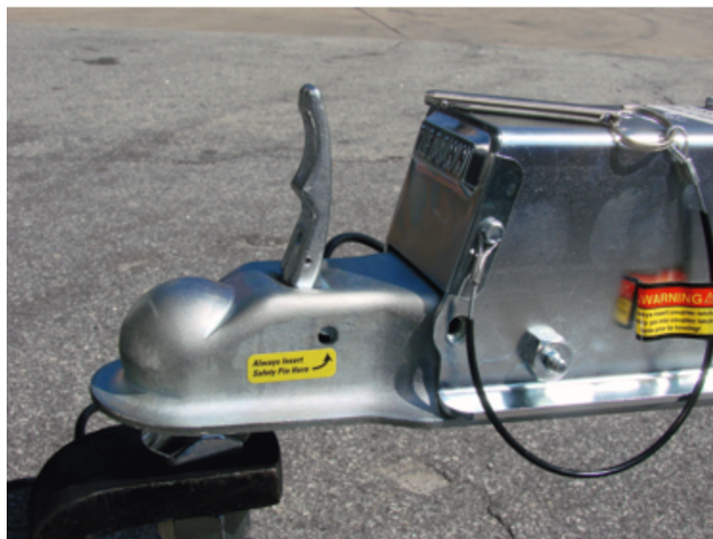
Photo A – Latch Open, Pin Not Installed
